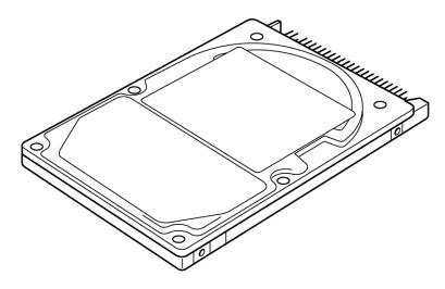
Figure 1-5 2.5-inch HDD
